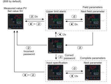
**5.2 Auto-tuning Process Flow** If the control mode Ctrl adopts APID or nPID mode, the PID parameters can be determined by auto-tuning. When the measured value PV is room temperature, please set the set value SV (parameter SP1) to about 60% of the commonly set temperature (for signals such as pressure or flow, it can be directly set to the commonly used set value), Pressand hold
